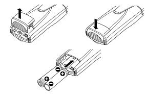
IMPORTANT — The batteries supplied with this product are rechargeable Ni-MH, 1300mAh. When replacing batteries, never use other types of batteries or conventional alkaline batteries.
