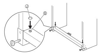
**13.** Tighten the screws you loosened in step 10 to secure the corner brackets to the side panels.
