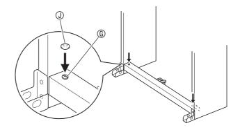
**13.** Secure the corner brackets to the stand using the screws you removed in step 10.
