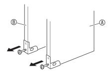
11. As shown in the illustration, reverse the corner brackets you removed in step 10, and insert pedal unit brackets ①-(a) and ①-(b) between the each of the corner brackets and the side panels ⓐ and ⓐ.
