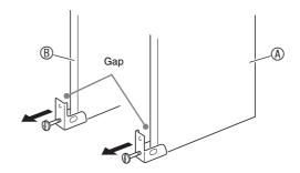
As shown in the illustration, insert the pedal unit brackets into to the gaps you created in step 10.
