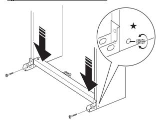
The side panels have joint connectors inside that engage with the corner bracket screws. If you have trouble inserting the screws into the joint connector screw holes, use a screwdriver to rotate the joint connector and adjust the position of the screw hole for easier access. See the detail drawing (marked with a star) in the above illustration.
