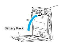
② Rotate the battery lock clockwise to secure the battery pack in place.
