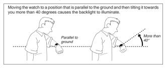
The backlight may not illuminate if the face of the watch is more than 15 degrees off the parallel as shown below. Make sure that the back of your hand is parallel to the
