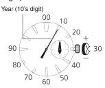
5. Rotate the crown to move the second hand to the desired setting for the year ten's digit.
