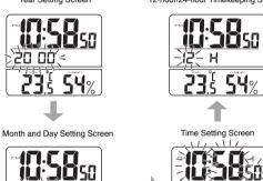
2. While the screen you want is on the display, use the Time Set buttons (1) to change the digits that are flashing.
