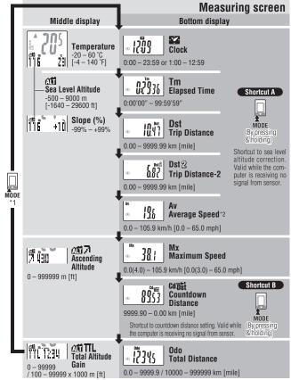
\*1 With the computer installed on the bracket, press on the four raised dots on the face of the computer. \*2 If **Tm** exceeds approximately 27 hours or **Dst** exceeds 9999.99 km, **.E** (Error) is displayed as the average speed. Reset data.
