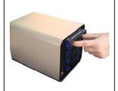
The tool-less drive-bays are designed to be secure and have as few parts as possible. However, accomplishing this requires that the user have a strong grasp! To remove the drive bays, pinch the front handle firmly until you are able to compress the blue plastic levers inside.
