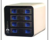
The CADA-U3E4 is designed to be hot-swappable. But if you have already setup an active 4-disk array, be careful not to insert any new drives. The automatic rebuild function will incorporate any new drives into the existing array. That means any existing data on the new drive will be wiped clean to accommodate the active array!
