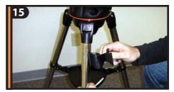
Attach plastic hand control holder to the tripod leg.
