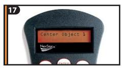
The hand control will prompt you to center the bright alignment star in the center of the eyepiece. Once centered, press ALIGN. This will accept the star as your first alignment position.
