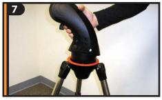
Hold the telescope fork arm and place the bottom of the base inside the tripod mounting platform as shown.
