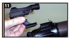
To attach the finderscope, loosen the silver screw and slide finderscope into mounting platform.
