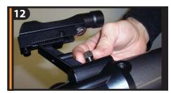
Secure finderscope to mounting platform by tightening the silver screw. The glass window of the finderscope should be facing towards the front of the telescope.
