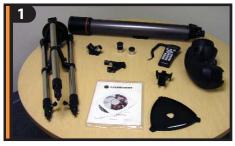
Your NexStar 80SLT includes: optical tube; fork arm; pre-assembled tripod; computerized hand control; hand control holder; star diagonal; two eyepieces; finderscope; accessory tray; documentation including an owner's manual, The Sky® CD and NSOL Telescope Control Software.
