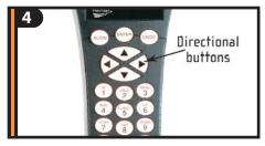
Use the hand control direction arrow buttons to point telescope at a distant land object, like a telephone pole or at night you can use the moon. Center and focus the object in the 25mm eyepiece of the telescope.
