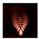
Please note: The larger the diameter of the main mirror and the shorter the focal length of the optical system, the more the telescope is affected by a small loss of collimation.
