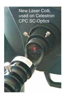
The alignment procedure itself is exactly the same as for a Newton optics – only much simpler.
