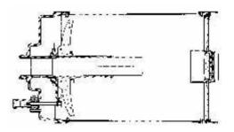
Simplified sketch of the SC-secondary mirror tilting mechanism. Three screws are arranged 120° apart, around a center pin on which the secondary mirror pivots.
