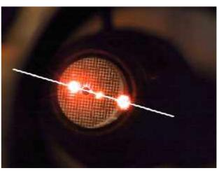
Having the reflected laser beam showing safely on the grid plane you can finish the collimation process quickly.
