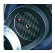
If you see this on your reference plane, adjust (tilt) your main mirror in a way that the laser point passes exactly through the center hole thus being reflected into itself.
