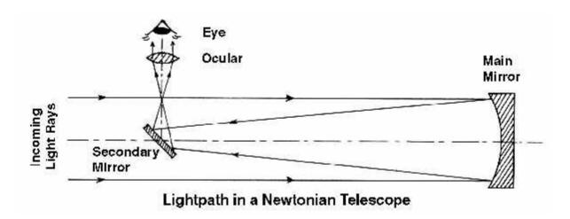
**The incoming light** travels first from left to right to the main mirror at the end of the tube, is reflected there and travels right to left, to the secondary mirror, which in turn deflects the light out of the tube and – via the eyepiece – into your eye.
