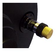
When there is only about 1/4" left to go, simply push the focuser the rest of the way in. This will take up some of the change in focus from when you removed the original focuser, making it quicker to return to focus the first time you use your telescope after the SCT MicroFocuser installation.
