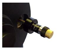
Begin threading the SCT MicroFocuser onto the threaded focus rod.
