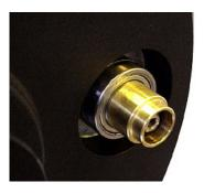
Use screwdriver to remove three screws from the focus assembly cover plate (the three screws around the outside of the focus shaft). Remove the cover plate. Hang on to the three Phillips screws as they will be used to attach the SCT MicroFocuser.
