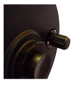
NexStar 11 GPS telescopes have a rubber knob which can be pulled off. Older 11" telescopes will have a metal focus knob which must be removed using a 1/16" hex-head wrench to loosen a small set screw. Once the knob is removed you will see the brass focus shaft as shown below.
