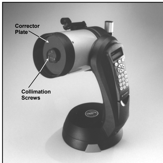
Figure 7-1 The three collimation screws are located on the secondary mirror holder in the center of the corrector plate.
