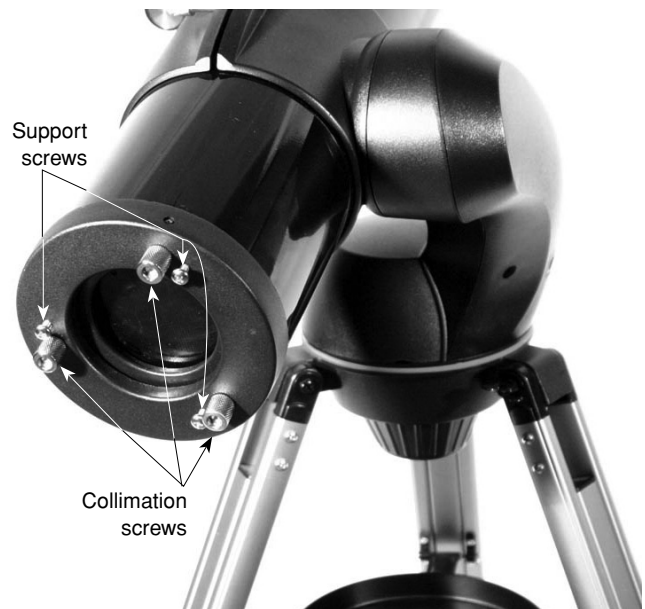
Figure 6-2. Collimation adjustment screws for the StarSeeker 114mm and 130mm.
