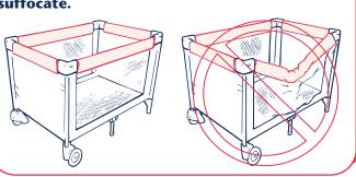
**5** Push down on center of Playard floor until it is flat and *locks* into position.
