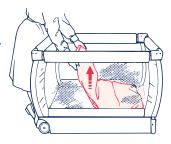
**4** Press release buttons on each hook and push hook into larger tube.
