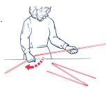
3 Slide rod completely into canopy fabric.
