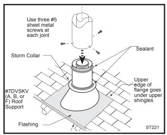
Fig. 31 Roof support and flashing.
