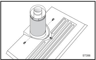
Fig. 21 Simpson Dura-Vent - install outer adapter pipe.
