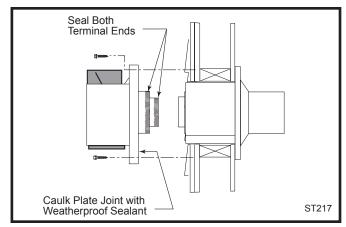
Fig. 27 Install the vent terminal.
