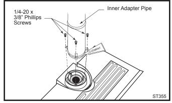
Fig. 20 Simpson Dura-Vent - install inner adapter pipe.
