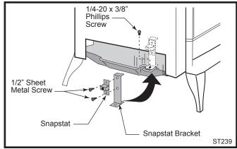
Fig. 13 Snapstat assembly and installation.
