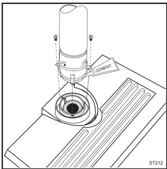
Fig. 18 Attach inner assembly to flue collar.
