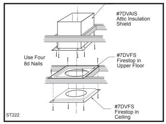
Fig. 30 Install firestops and attic insulation shield.
