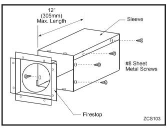
Fig. 23 Assemble the wall sleeve and firestop.
