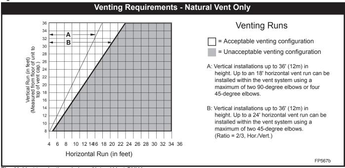
Fig. 11 Vent termination window - Natural Vent ONLY.
