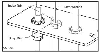
Fig. 55 Remove pilot orifice.
