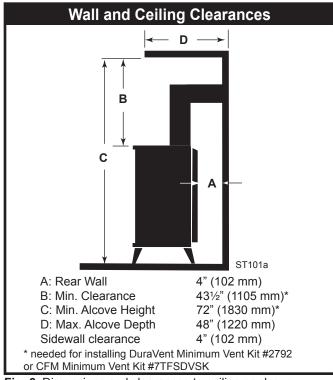
Fig. 6 Dimensions and clearances to ceiling or alcove.
