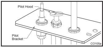
Fig. 54 Remove pilot hood.
