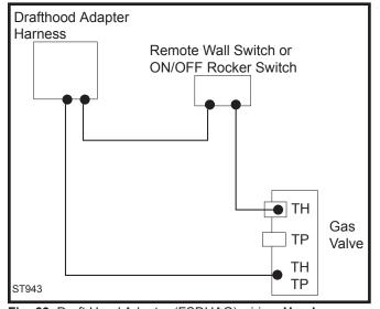
$\label{eq:FSDHAG} \textbf{Fig. 63} \ \ \text{Draft Hood Adapter (FSDHAG) wiring. } \textbf{Used on RN/RP models only.}$
