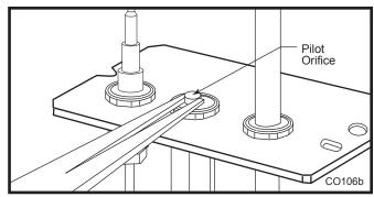
Fig. 57 Remove pilot orifice.
