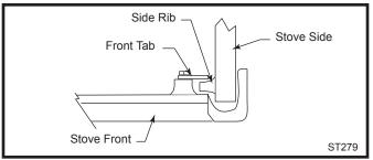
Fig. 45 Engage with side ribs
