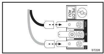
Fig. 43 Attach switch wires to valve.
