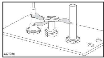
Fig. 49 Correct pilot flame pattern. SIT valve.
