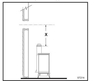
Fig. 24 Determine the vertical pipe length.
