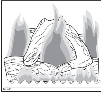
Fig. 50 Correct burner flame appearance.
