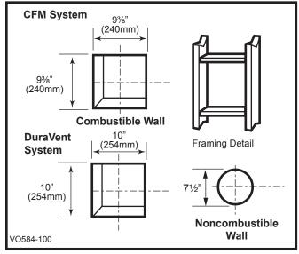
Fig. 22 Locate vent opening.
