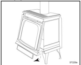
Fig. 59 Remove the Stove Front.
