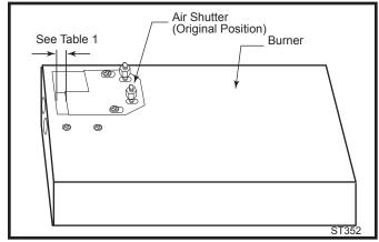
Fig. 39 Air shutter in original from-the-factory position.
