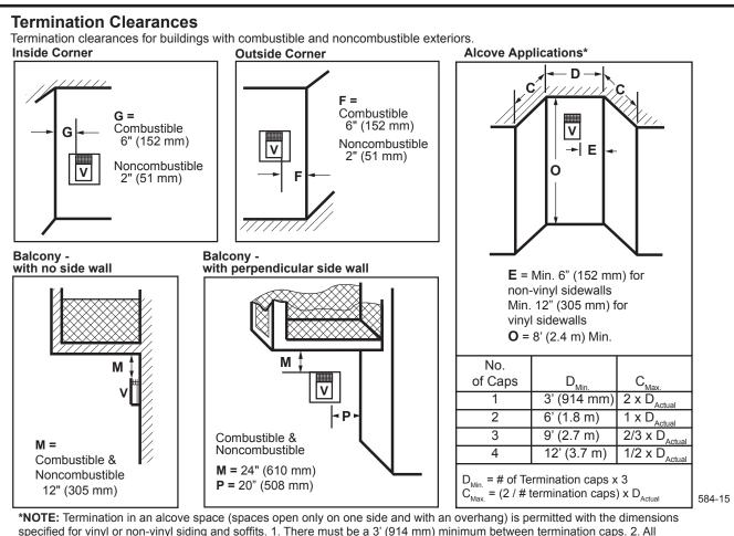
\*NOTE: Iermination in an alcove space (spaces open only on one side and with an overhang) is permitted with the dimensions specified for vinyl or non-vinyl siding and soffits. 1. There must be a 3' (914 mm) minimum between termination caps. 2. All mechanical air intakes within 10' (1 m) of a termination cap must be a minimum of 3' (914 mm) below the termination cap. 3. All gravity air intakes within 3' (914 mm) of a termination cap must be a minimum of 1' (305 mm) below the termination cap.
