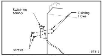
Fig. 42 Attach switch assembly to rear shroud.
