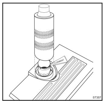
Fig. 33 Install draft hood adapter.
