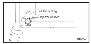
Fig. 58 Remove and replace injector orifices.
