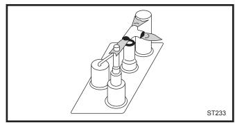
Fig. 48 Correct pilot flame appearance. PSE pilot.
