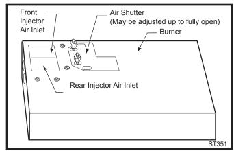
Fig. 40 Air shutter adjusted.
