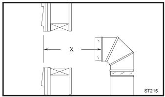
Fig. 25 Measure the horizontal length.
