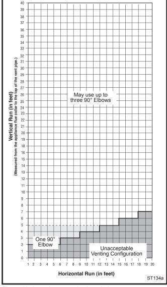
Fig. 7 Horizontal vent termination window.
