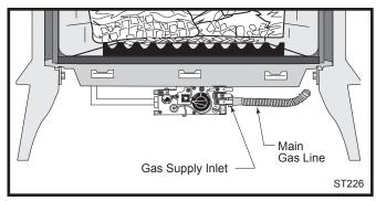
Fig. 51 Attach the gas line to the left side of the valve.
