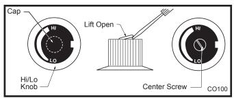
Fig. 52 Remove center screw from Hi-Lo knob.
