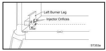
Fig. 41 Remove and replace injector orifices.
