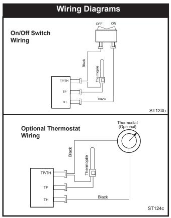
Fig. 62 On/off switch and optional thermostat circuit.
