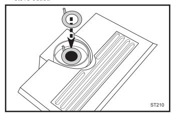
**Fig. 16** Install the restrictor plate only if required for the venting configuration. Refer to Page 9.
