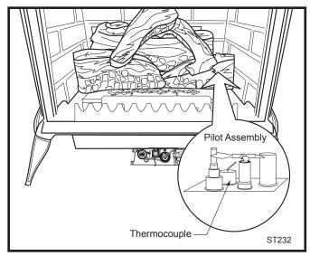
Fig. 46 Pilot assembly location.
