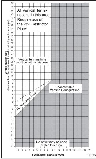
Fig. 8 Vertical vent termination window.
