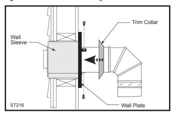
Fig. 26 Install the horizontal pipe and wall plate parts.
