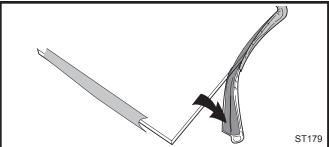
**Fig. 61** Wrap the gasket material around the outside edge of the glass. 30004177
