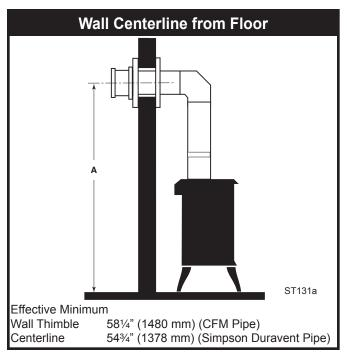
Fig. 5 Minimum wall thimble centerline.
