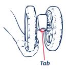
**2** Tilt stroller slightly back and push wheel assembly onto leguntil it *locks* in place.
