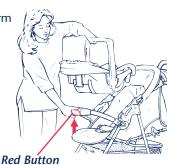
4 After removing car seat, insert Tongue of arm bar pad into arm bar Slot.
