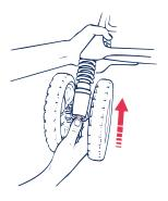
**CAUTION:** After wheel assembly is complete, pull on wheels to check that they are *locked* in place.
