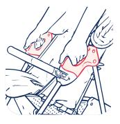
**6** Engage latch on side of stroller to retain stroller in locked position.
