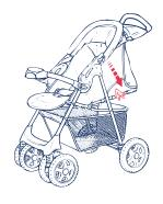
With car seat handle in *locked* carrying position (upright) insert car seat adapter *Tongue* into arm bar *Slot*.
