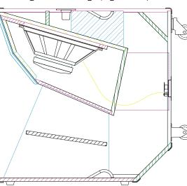
require a long horn. The challenge to reduce the horn's dimensions without decreasing its length results in a technique that involves "folding" the horn. This technique collapses the physical dimensions of the horn without reducing
