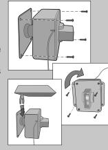
**Vehicle Alert Installation:** For cars, the best mounting position is about 4 feet (1.2 m) high, between 10-20 feet (3-6 m) back, and angled to see the back of car after passing the sensor.
