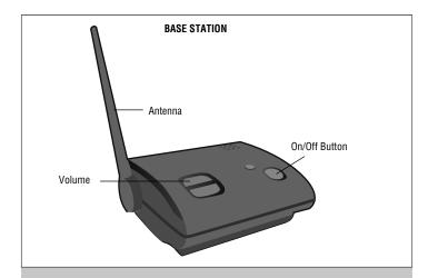
**On/Off:** To turn the Base Station on and off, hold down the power button until you hear the on/off tone.
