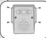
Mount PIR Motion Sensor vertically on solid surface a few feet off the ground and within 1000' of Base Station. Unit should be able to swivel as needed.
