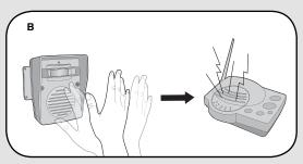
**B** Within 5 seconds, wave hand in front of PIR Motion Sensor. Test light will illuminate and Base Station will activate with static and feedback after several seconds.
