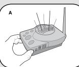
A Ensure that Base Station and PIR Motion Sensor are in close proximity to each other. Press and release learn button on Base Station. Buzzer will sound.
