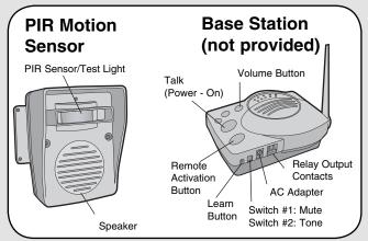
**On/Off:** To turn Base Station OFF hold down the Volume button until a beep is heard and light goes out. To turn Base Station ON press the Talk button.
