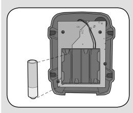
Install 4 AA Alkaline batteries (not provided). (Lithium batteries recommended for colder environments.) Keypad will beep.
