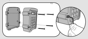
Mount the Keypad onto the back panel with screws. Tighten screws with Allen wrench.
