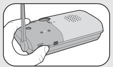
Press the Learn button on the new intercom until a beep is heard. Within 10 seconds put the second intercom into Learn Mode (refer to the following table).
