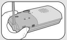
Press the Learn button on the new intercom until a beep is heard. Within 10 seconds put any networked intercom into Learn Mode (refer to table below).
