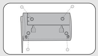
Adhere rubber pads to bottom. Repeat Steps 1 and 2 for any additional intercoms.
