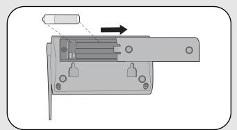
Install 4 AA Alkaline batteries (not provided). (Lithium batteries recommended for colder environments.)
