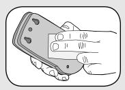
Clean back of intercom and mounting surface using the alcohol wipe.
