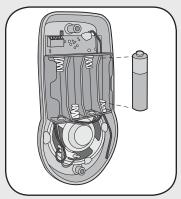
Install 4 AA Alkaline batteries (not provided). (Lithium batteries recommended for colder environments.)
