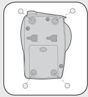
**Step 2:** Adhere rubber pads to bottom. Repeat Steps 1 and 2 for any additional intercoms.
