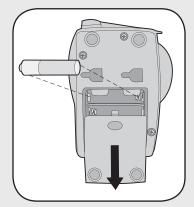
**Step 1:** Install 4 AA Alkaline batteries (not provided). (Lithium batteries recommended for colder environments.)
