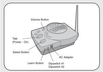
**On/Off:** To turn Indoor Intercom ON, press any button. To turn Indoor Intercom OFF, hold down the Volume button for 5 seconds.
