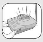
Step 2: Within 10 seconds press the Learn button on the Outdoor Intercom until a multi-beep is heard. *NOTE:* The Indoor Intercom will beep for approximately 30 seconds indicating that programming is successful. To stop the beeps earlier, press the Select Button on the Indoor Intercom.
