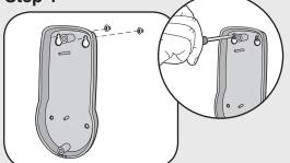
Mount Outdoor Intercom with small silver screws. Screw the top two screws halfway into the mounting surface. Place back of Outdoor Intercom over screws. Tighten screws.
