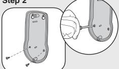
Put the remaining silver screws into the bottom holes of Outdoor Intercom. Tighten screws.
