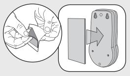
Peel off white paper from mounting tape. Firmly press mounting tape on back of Outdoor Intercom.
