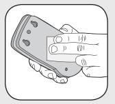
Clean back of Outdoor Intercom and mounting surface using the alcohol wipe.
