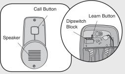
**Call Button:** To communicate with the Indoor Intercom, press and release the Call button. A doorbell sound will be heard on the Indoor Intercom. Once a secure link is made, the Call button on the Outdoor Intercom does not need to be pressed to speak again.
