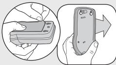
Peel paper from mounting tape. Firmly press Outdoor Intercom onto mounting surface.
