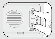
Press and hold both buttons on the intercom for 5 seconds. An initial beep will be heard followed by a second beep. The channel lights will flash. Within 10 seconds put the second intercom into Learn Mode (refer to table below).
