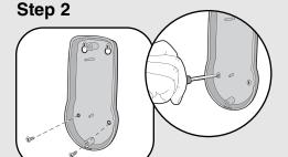
Put the remaining silver screws into the bottom holes of intercom. Tighten screws.
