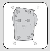
Adhere rubber pads to bottom. Repeat Steps 1 and 2 for any additional intercoms.
