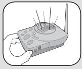
Press the Learn button on the new intercom until a beep is heard. Within 10 seconds put any networked intercom into Learn Mode (refer to table below).
