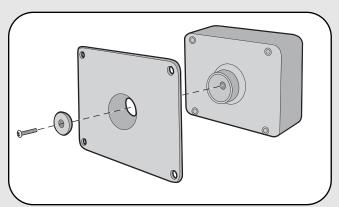
Attach PIR Motion Sensor box to mounting plate with large silver screw. Tighten screw until PIR Motion Sensor stays in place when repositioned.
