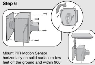
of Base Station (rotate sensor to access screw holes). Unit should be able to swivel as needed. Attach sun/rain shield.
