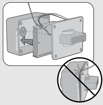
Insert battery pack facing away from circuit board and attach cover.
