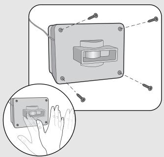
Test PIR Motion Sensor by waving hand in front of sensor. Test light should flash. Secure cover with the smallest screws.
