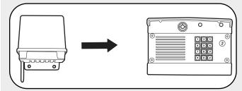
**Step 1:** On the phone connected to the OTIUEX, press "\*\*07" after hearing the dial tone. Listen for a double beep. Hang up and Learn LED will flash for 15 seconds. If an error tone is heard it means that memory will have to be cleared (see Troubleshooting).
