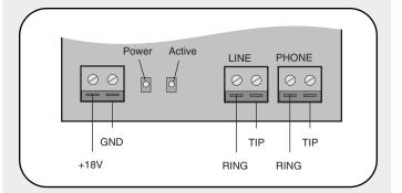
Use the supplied Test/Program Cord for programming and testing before completing connections to phone company's d-mark box.
