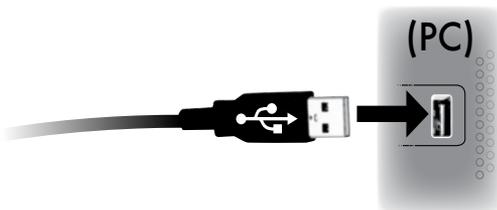
**5** USB functions on the display unit are OFF by default. Verify the display unit is powered on and receiving data from the outdoor sensor. Next, set the USB mode on the display unit. Set to mode 3 for full PC Connect functionality, or see page 5 for a description of all available USB modes.
