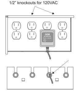
The H290 provides space for 4 standard duplex receptacles. Wires should exit the H290 using the grommets provided. The grommets may be cut as shown.
