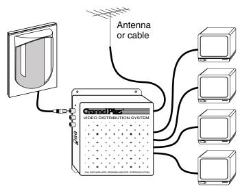
Using an All in One Video Distribution System such as a ChannelPlus model 3015, you may view the camera on an unused UHF or cable channel. (For example, the front door camera could be UHF channel 50. All antenna channels will appear normal.)
