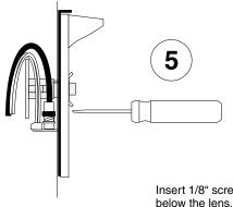
Insert 1/8" screwdriver in the steering slot below the lens. Using the screwdriver, bend the mount to point the camera in the desired direction. Never use the camera to bend the mount!
