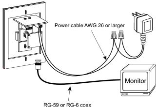
RG-59 or RG-6 coax A long cable run (150ft or more) can noticeably reduce the picture brightness and increases the possibility of ground loop hum.
