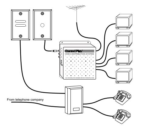
A ChannelPlus DoorTel system (model 9400) is an ideal addition to this system. In this house, when the doorbell rings, the homeowner changes the TV to the front door channel and picks up any phone in the house. The homeowner can talk with and see the guest at the front door.
