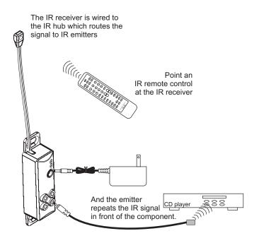
Be sure the emitter is attached directly over the component's IR receiver. To locate the IR receiver, shine a flashlight into the unit and look for the
