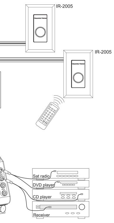
The diagram above illustrates how to create an IR system with IR receivers in several different rooms in the house. Systems like this may include several different
