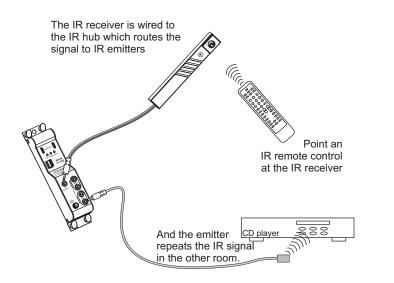
Be sure the emitter is attached directly over the component's IR receiver. To locate the IR receiver, shine a flashlight into the unit and look for the sensor.
