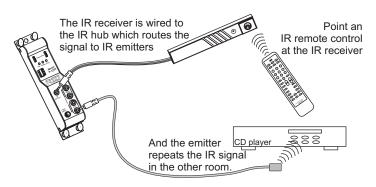
Be sure the emitter is attached directly over the component's IR receiver. To locate the IR receiver, shine a flashlight into the unit and look for the sensor.
