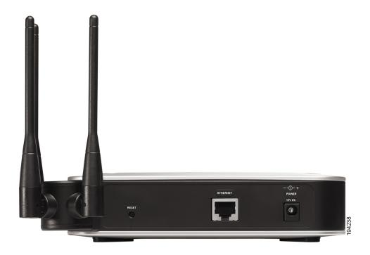
**RESET Button**—There are two ways to reset the access point to the factory default configuration. Either press the Reset button for approximately 10 seconds or restore the defaults using the web-based utility of the access point.
