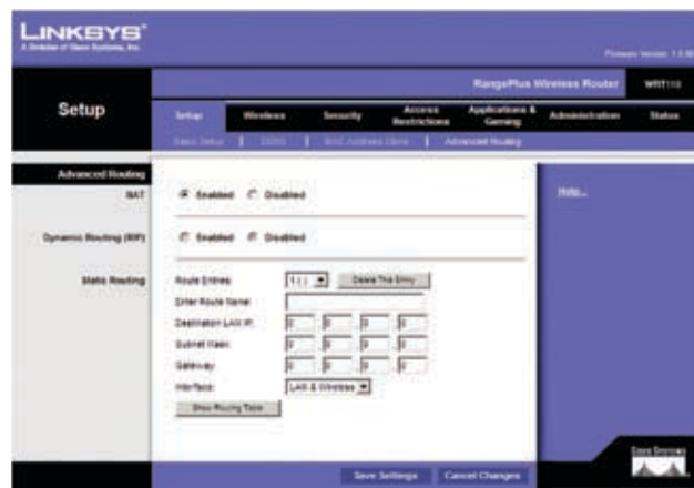
Setup > Advanced Routing
