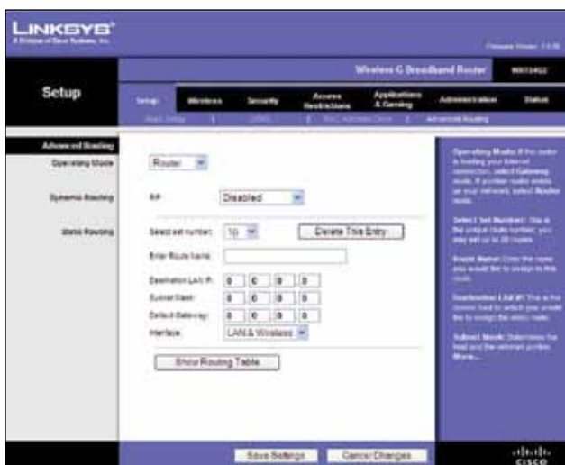
Setup > Advanced Routing (Router)
