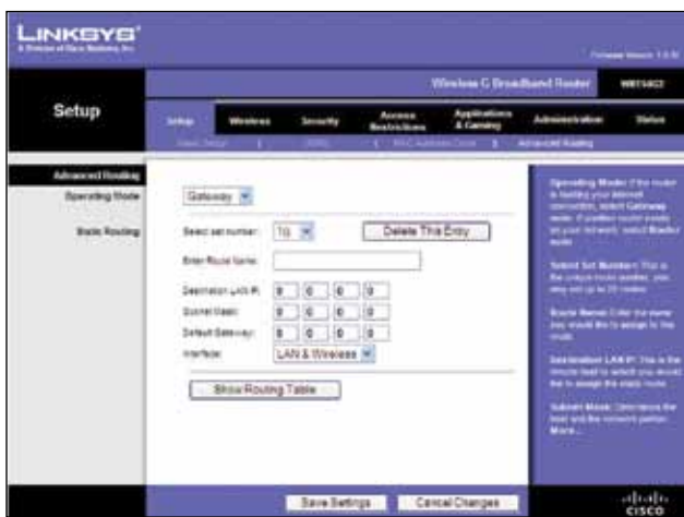
Setup > Advanced Routing (Gateway)
