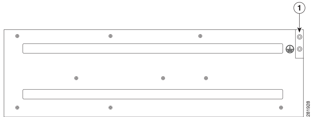
Figure 3-7 Attaching a Grounding Lug to the Rear of the Router
