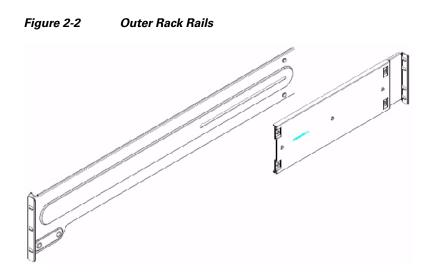
**a.** Make sure that the right short and long outer rack rail brackets are connected to each other and that the left short and long outer rack rail brackets are connected to each other.
