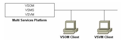
A single site deployment can include many Multi Service Platforms. In this situation, VSOM runs on one Multi Service Platform, either by itself or with other VSM software. The other Multi Service Platforms run VSMS. A deployment of this type allows scaling the solution to address wiring requirements and to support a large number of cameras and increased retention rates.
