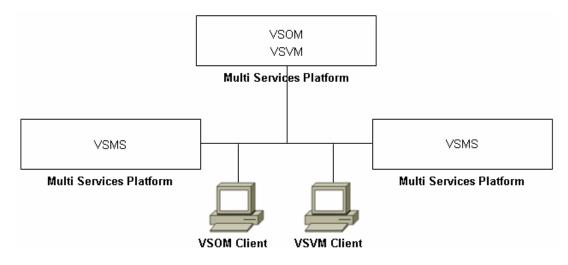
Figure 1-2 Single Site Deployment with Several Multi Services Platforms
