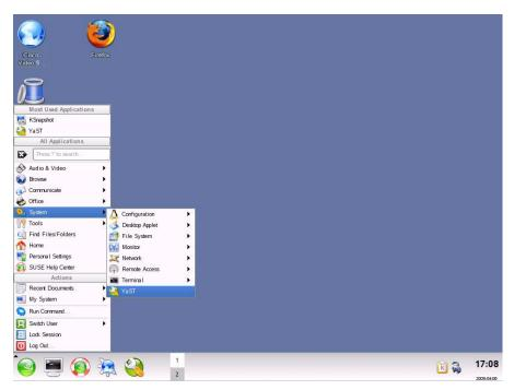
Figure 2-5 Accessing the YaST Control Center
