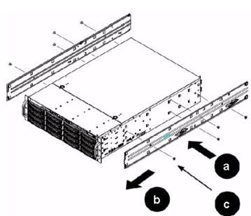
Figure 2-1 Attaching Inner Rack Rails
