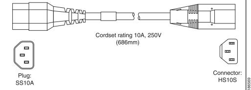
Figure B-14 CAB-C13-C14-2M, Jumper Power Cord (2 m)
