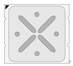
**d.** For a new heatsink, peel the protective film from the thermal pad that is on the bottom of the new heatsink.
