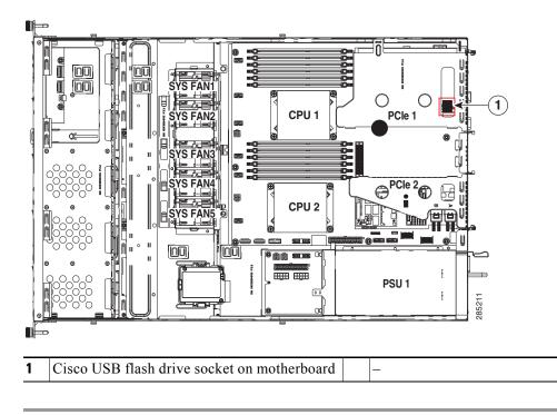
Figure 3-22 Internal USB Flash Drive Socket (USB 2.0)
