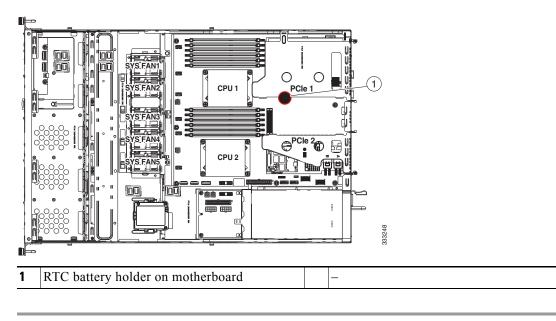
Figure 3-18 Replacing the Motherboard RTC Battery
