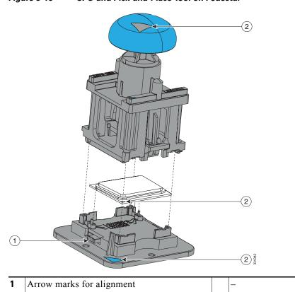
Figure 3-16 CPU and Pick-and-Place Tool on Pedestal
