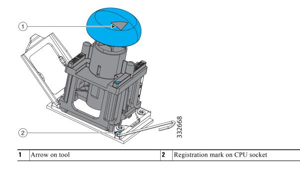
**Step 4** Insert the new CPU into the Pick-and-Place tool:
