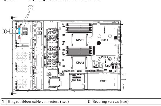
Figure 3-8 Replacing the Front Operations Panel Board
