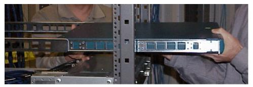
Figure 1-5: Sliding the Switch Into the Rack
