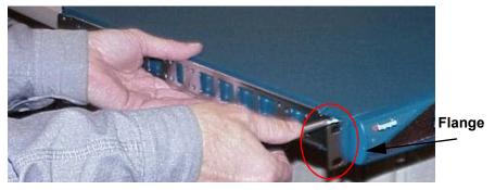
Figure 1-2: Attaching One Rail to Server Switch Chassis
