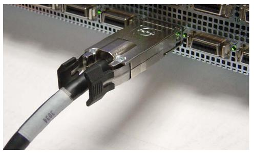
Figure 1-7: Fully Installed IB Cable with Pinch Connector
