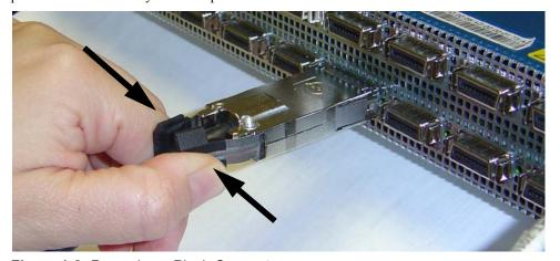
Figure 1-8: Removing a Pinch Connector
