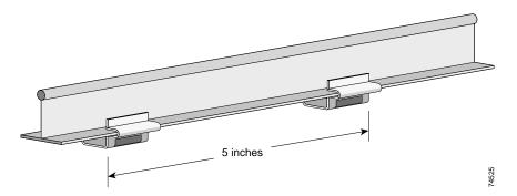
Step 6 Grasp the antenna with one hand and the track with the other while inserting the antenna's mounting clips into the ceiling mounting clip adapter until they can go no further as shown in the following illustration.
