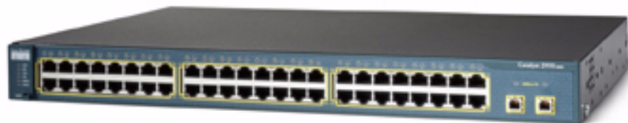
Figure 5 Cisco Catalyst 2950SX-48 Switch
