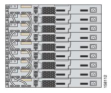
In this example, the stacks use both the 0.5- and the 3-meter StackWise cables to make redundant connections.
