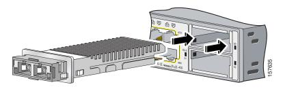
When installing a transceiver module or the Cisco TwinGig Converter Module in the upper 10-Gigabit Ethernet module slot (slot 1), position the module face up. When using the lower module slot (slot 2), position the module face down.
