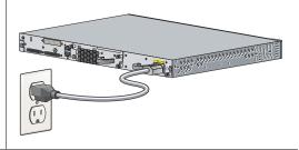
**Step 3** When the switch powers on, it begins the power-on self-test (POST). During POST, the LEDs blink while tests verify that the switch functions properly.
