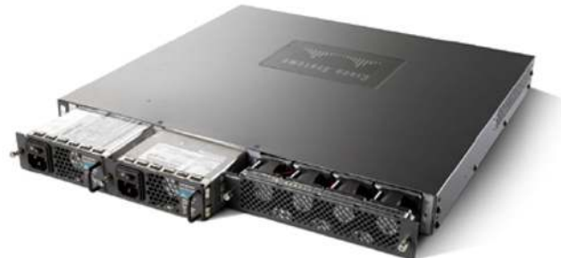
Figure 2. Rear View of Cisco Catalyst 4948 with Dual Redundant Power Supplies and Removable Fan Tray
