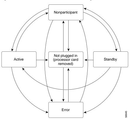
Figure 3-1 CPU Switch Module State Transition Diagram
