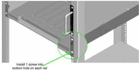
Step 5 On each side of the chassis, install a screw and caged nut into the holes above and below the handle.
