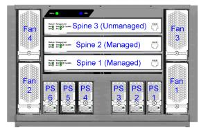
Figure 2-9 SFS 7012 Chassis – Spine Module Slot Numbering
