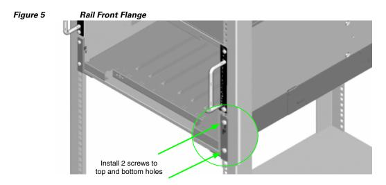
Install the second rail on the other side of the rack by repeating steps 1 through 3.
