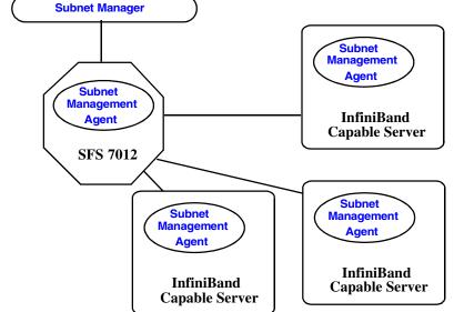
The Subnet Manager utilizes the agent information to discover and manage connections from the SFS 7012 to the InfiniBand fabric. The Subnet Manager maintains a database tracking subnet topology information as a result of its interaction with the SMAs.
